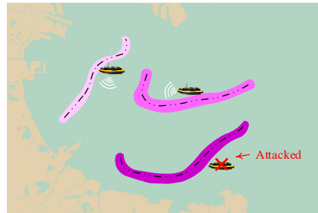
Fig. 1. Case study of monitoring a marine environment with aquatic robots. The robots are tasked with finding informative paths to gather data. The darker the color of path is, the more valuable path since it gathers information from a more important region. We investigate the question of how the robots should plan their paths if we expect some of the robots to fail due to adversarial elements or natural causes?
