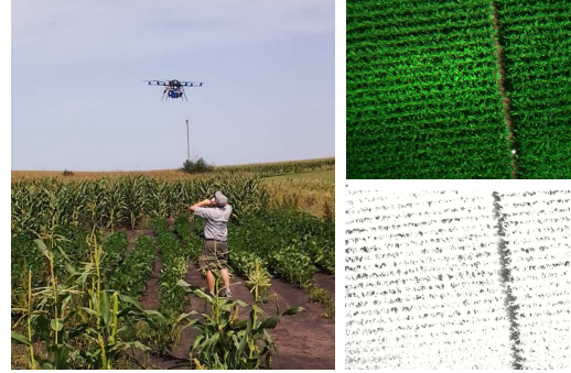
Fig. 11. Preliminary field experiment with a UAV carrying a multi-spectral camera in a corn plot in Janesville, MN, U.S.A. Visible and near-infrared images shown were obtained from an altitude of 30 m during the experiment.
