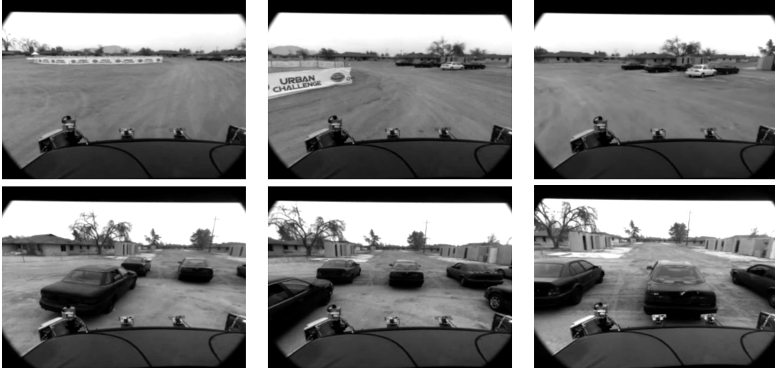
Fig. 1: Caltech’s entry Alice in the 2007 DARPA Urban Challenge undergoing a qualifying test. Top row : Alice entering the lot and navigating to parking spot, Bottom row : Multiple attempts to pull-in to spot before successful parking. Alice’s requirement, or system specification , is to safely park in a parking spot. Informally, one possible test specification could be that Alice should require more than one attempt in entering the parking spot to successfully park. Given an empty parking lot as the original test environment, how should obstacles be placed such that Alice requires more than one attempt (satisfying the test specification ) to successfully park (satisfying the system specification )? The locations of obstacles was manually decided in this test; how can we automate finding constraints on the test environment?
