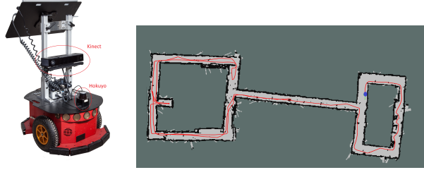
Fig. 9. (Left) Pioneer P3-DX with the Hokuyo laser used for the experiments. The 2D Hokuyo laser was used for robot localization and the Kinect2 sensor was used for mapping during exploration. (Right) Final map as well as the exploration path during the corridor experiment.
