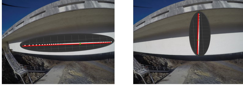
Fig. 3 White dots: LIDAR data; Red line: best fit using Hough Transform.
